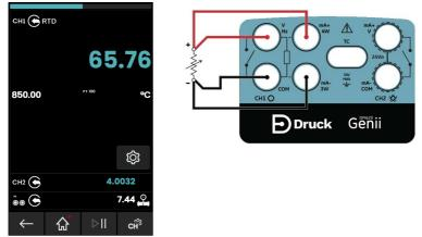
Figure 4-12: PT100 RTD Measure CH1 4-Wire (Range -200 to 850°C)
