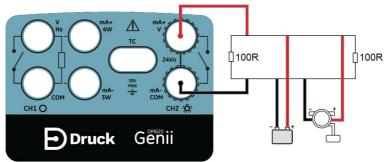
Figure 10-1: Example Connection Diagram FOUNDATION™ Fieldbus
