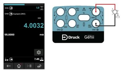
Figure 4-8: Measure Current on CH2 with Internal Loop Power (Range: 55mA)
