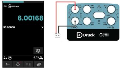
Figure 4-2: Measure DC Volts or DC mV on CH1 (Range ± 30V)
