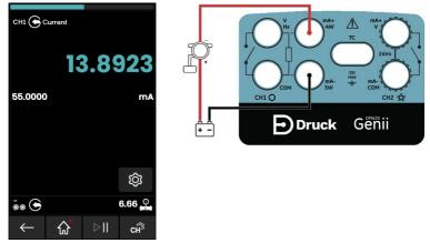
Figure 4-1: Measure Current on CH1 (Range ± 55mA)
