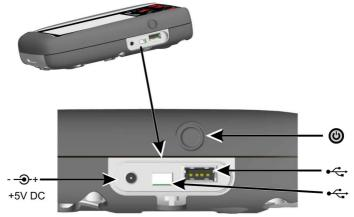
Figure 1-4: DPI620G Power Button and Ports
