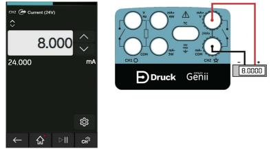
Figure 4-7: Source Current on CH2 with Internal Loop Power (Range: 0 to 24mA)
