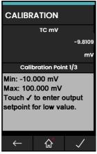
Figure 12-10: Calibration – TC mV Measure CH1 (Range: ± 100 mV)
