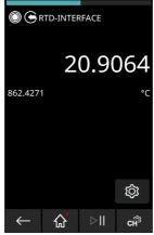
Figure 6-5: Example: RTD-INTERFACE on External Sensor Channel
