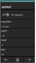
**OUTPUT** relates to the output signal from the Device Under Test (DUT). When the screen shows the wanted parameter values, tap on the  $\rightarrow$  icon to show the **TOLERANCE** screen.
