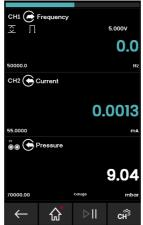
Figure 3-1: Calibrator Window – Normal View (Three Channels)
