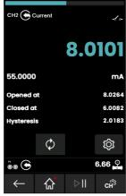
Figure 3-18: Switch Test Example
