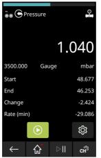
Figure 5-16: Example: Leak Test Results
