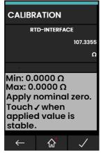
Figure 12-11: Calibration – RTD-INTERFACE
