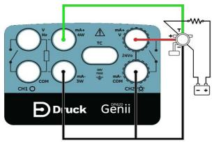
Figure 9-4: HART® Device Test Connections
