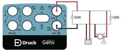
Figure 11-2: Example Connection Diagram Profibus®
