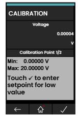
Figure 12-5: Calibration – Voltage Source CH1 (Range: 20 V)
