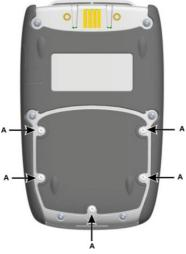
Figure 1-3: Installing the Battery
