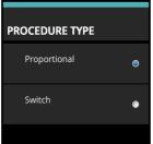
The display shows the INPUT parameters screen. If necessary, tap on a menu row to select it and change its value by the use of either a related onscreen keyboard or menu radio button.
