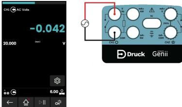
Figure 4-3: Measure AC Volts or AC mV on CH1 (Range  $\pm$  20V RMS)
