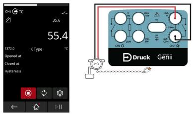
Figure 4-19: Thermocouple Switch Test
