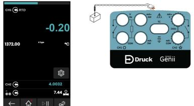
Figure 4-16: K-Type Thermocouple Measure CH1 (Range -270 to 1372°C)
