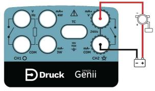
Figure 9-2: HART® Device Connection on CH2
