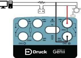
Figure 9-3: HART® Communicator Network Connection
