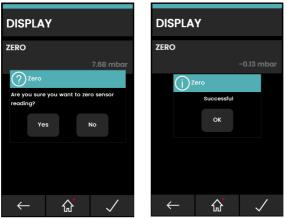
Figure 5-17: Pressure Module Zero Example
