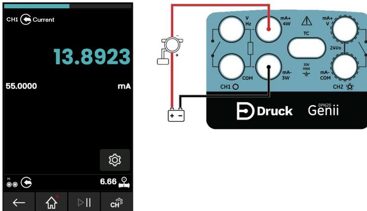
**Figure 4-1: Measure Current on CH1 (Range  $\pm 55$ mA)**
