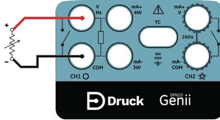
Figure 4-14: PT100 RTD Measure CH1 2-Wire (Range -200 to 850°C)
