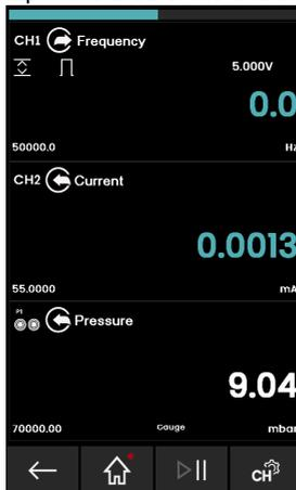
**Figure 3-1: Calibrator Window – Normal View (Three Channels)**
