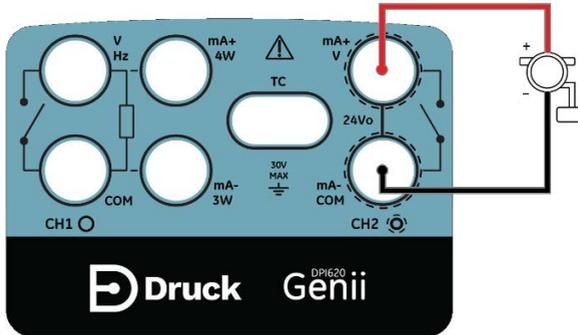
Figure 9-1: HART® Device Connection with Loop Power
