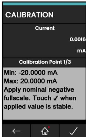
Figure 12-2: Calibration – Current Measure (Range: 20mA)
