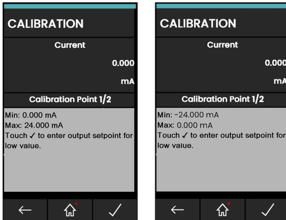
**Figure 12-3: Calibration – Current Source (Range: +24mA and -24mA)**
