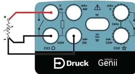
Figure 4-13: PT100 RTD Measure CH1 3-Wire (Range -200 to 850°C)
