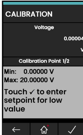
**Figure 12-5: Calibration – Voltage Source CH1 (Range: 20 V)**
