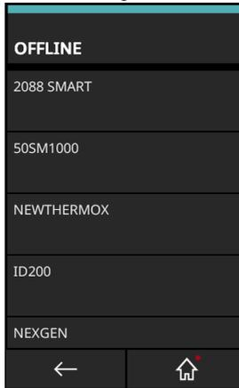
**Figure 9-18: HART® Offline – Saved Configuration Files Selection**
