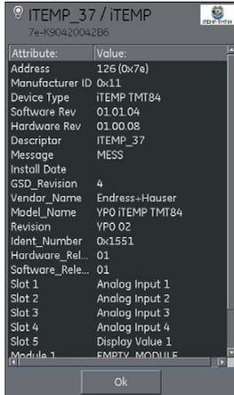
**Figure 11-10: Profibus® Device Profile**
