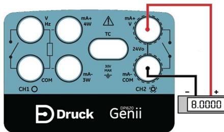
Figure 4-7: Source Current on CH2 with Internal Loop Power (Range: 0 to 24mA)
