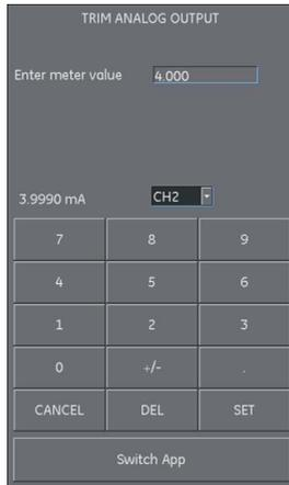
**Figure 9-29: Enter Calibration Point**
