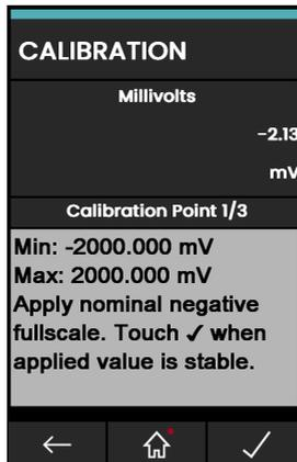
**Figure 12-4: Calibration – Millivolts Measure (Range:  $\pm 2000\text{mV}$ )**
