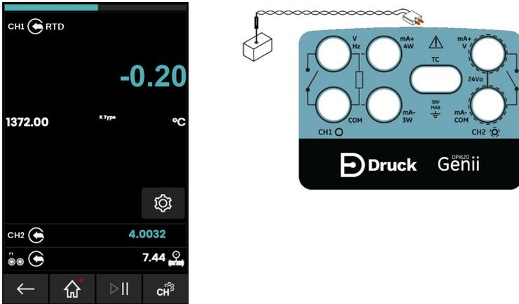
Figure 4-16: K-Type Thermocouple Measure CH1 (Range -270 to 1372°C)
