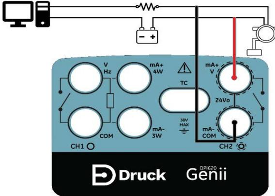
**Figure 9-3: HART® Communicator Network Connection**
