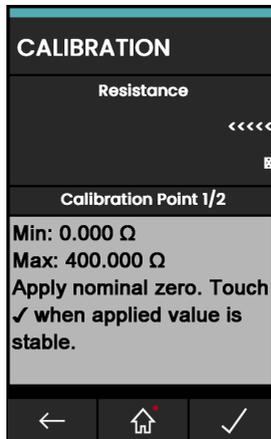
**Figure 12-8: Calibration – Resistance Measure CH1 (Range: 400Ω)**
