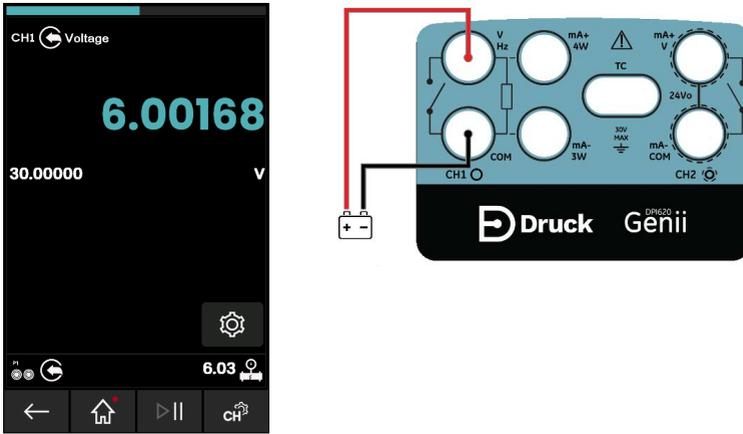
**Figure 4-2: Measure DC Volts or DC mV on CH1 (Range  $\pm 30V$ )**
