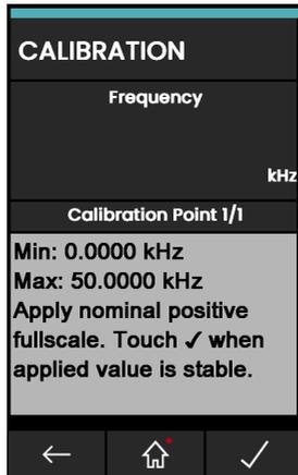
**Figure 12-6: Calibration – Frequency Measure CH1 (Range: 50 kHz)**
