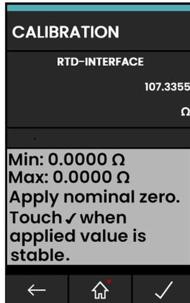
Figure 12-11: Calibration – RTD-INTERFACE
