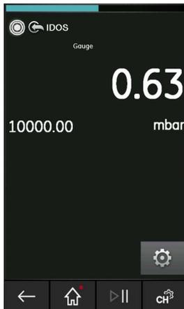
Figure 5-13: IDOS Pressure Measurement on External Sensor Channel
