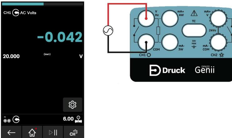
**Figure 4-3: Measure AC Volts or AC mV on CH1 (Range  $\pm 20V$  RMS)**
