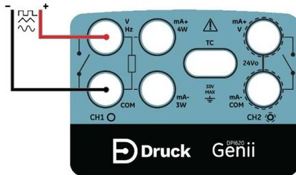
Figure 4-9: Example A – Measure Frequency on CH1 (Range 0 to 50kHz)
