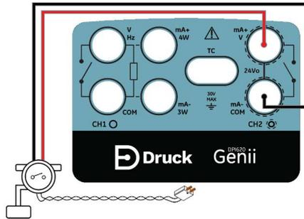
Figure 4-19: Thermocouple Switch Test
