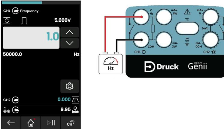
Figure 4-10: Example B – Source Frequency CH1 (Range 0 to 50kHz)
