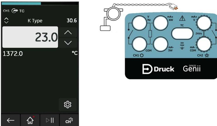
Figure 4-17: K-Type Thermocouple Source CH1 (Range -270 to 1372°C)
