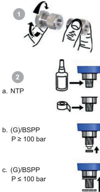
**Figure 5-8: Pressure Connections**
